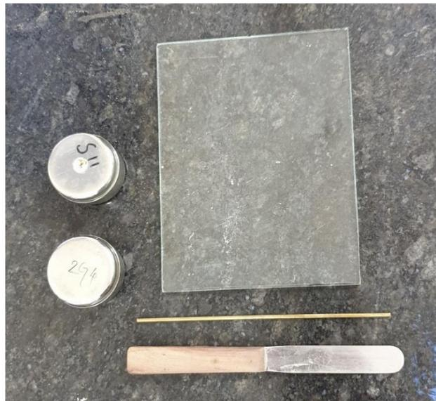
Figure 1: Equipment for Plastic Limit
