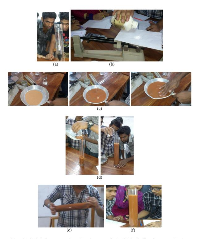
Figure 4.2: (a) Take the zero correction and meniscus correction (b) Weight the dispersion agent and make a water-agent solution. (c) Take powdered soil and mix with water-agent solution in a pan. (d) Pour the mixture at cylinder carefully (e) Shake very carefully (f) Place the hydrometer at the cylinder and take reading carefully
