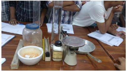
Figure 4.2 Hydrometer Test Apparatus
