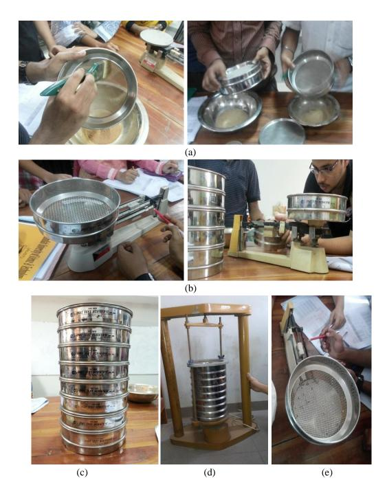
Figure 3.1: (a) Clean all seives before test. (6b) Weight all seives (c) Serially set all seives according to their opening size. (d) After pouring the soil place it to seive shaker and shake 10 min. (e) Weight all seive with contained soil
