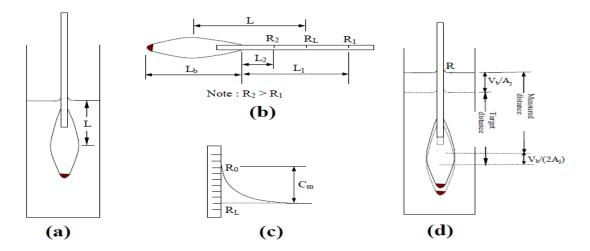
Figure 4.1 Schematic diagrams showing hydrometer readings and corrections.
