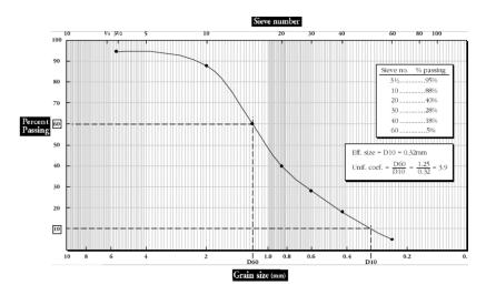
Figure 3.1: Gradation Curve (www.aboutcivil.org/Sieve-analysis-and-soil-classification.html)
