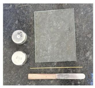
Figure 1: Equipment for Plastic Limit
