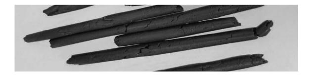
Figure 3: 3 mm thread of soil with cracks
