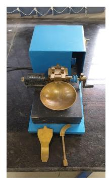
Figure 1: Casagrande's liquid limit device
