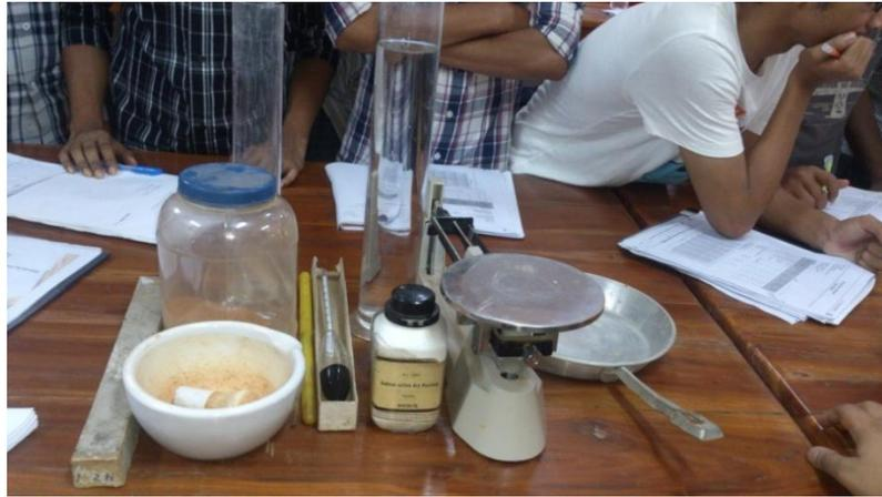
Figure 4.2 Hydrometer Test Apparatus
